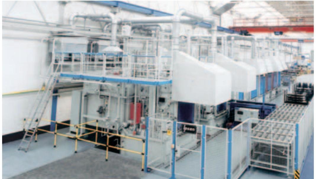
**Description** CARBOTHAN® is a nitrogen-methanol based atmosphere system, which generates a very flexible, high-quality atmosphere for carburising, neutral hardening, annealing and sintering of steel.
